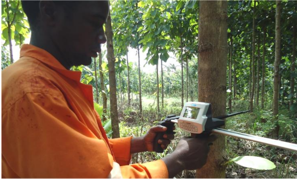
Figure 5: Diameter at Breast Height (DBH) measurement being conducted using Masser Calliper during an enumeration exercise
