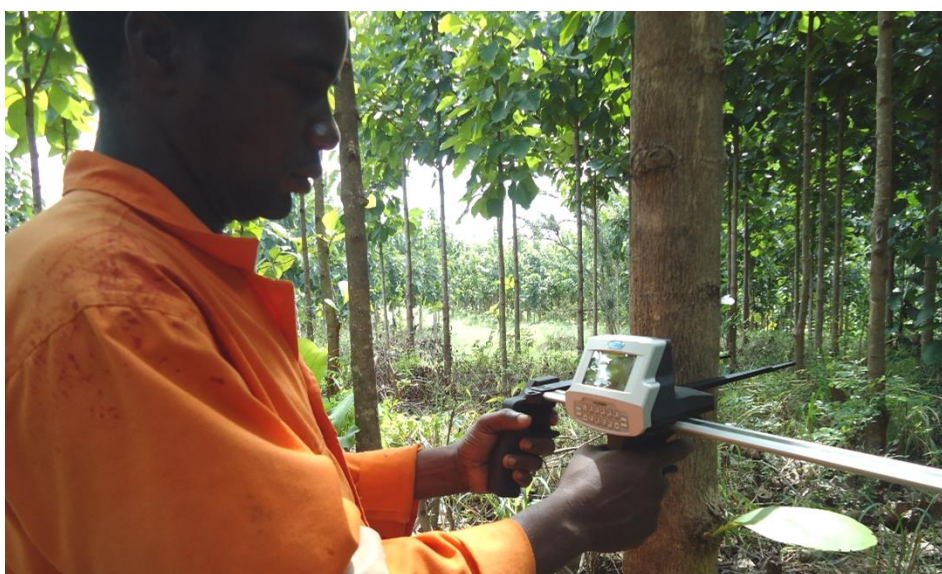
Figure 5: Diameter at Breast Height (DBH) measurement being conducted using Masser Calipers during an enumeration exercise
